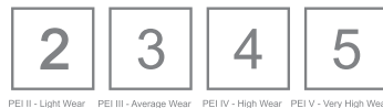
PEI II - Light Wear PEI III - Average Wear PEI IV - High Wear PEI V - Very High Wear
